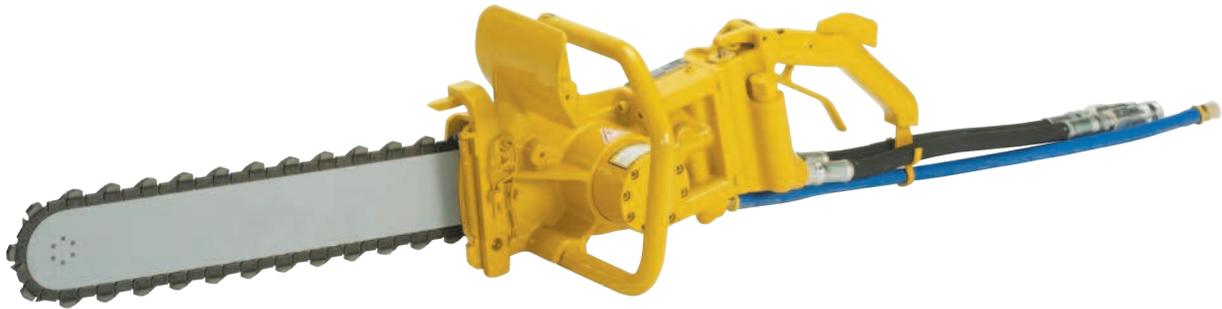
The **DS11** Diamond Chain Saw is specifically designed to cut solid concrete underwater. Cuts square corners without over-cut and can plunge cut sea walls up to 18" thick. Two available bar lengths (15" and 18") and two different chains depending on the amount of rebar and hardness of the concrete. A minimum of 20 PSI water pressure is required at the saw for cooling and lubrication of the bar and chain. Painted hi-visibility yellow.
